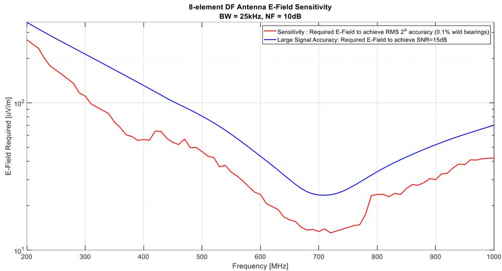
This plot indicates the electric field strength required to achieve a SNR of 15dB (blue line) and the E-field strength required to achieve an RMS error of 2° or better. This plot allows the customer to directly evaluate whether this antenna is appropriate for the type of signals expected in their specific application. Notice however, that these plots also require several assumptions (like the channel bandwidth and noise figure of the system), and these should be stated explicitly.
